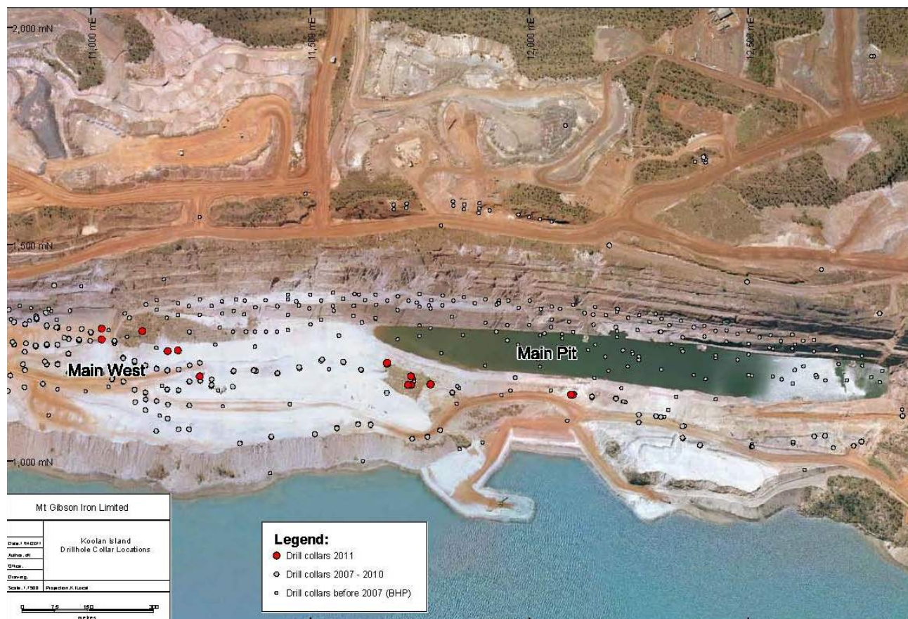
Figure 15 – Plan of Main Pit, Koolan Island showing drillhole collar locations for holes drilled during the quarter (red circles) and all previous drilling (grey)
