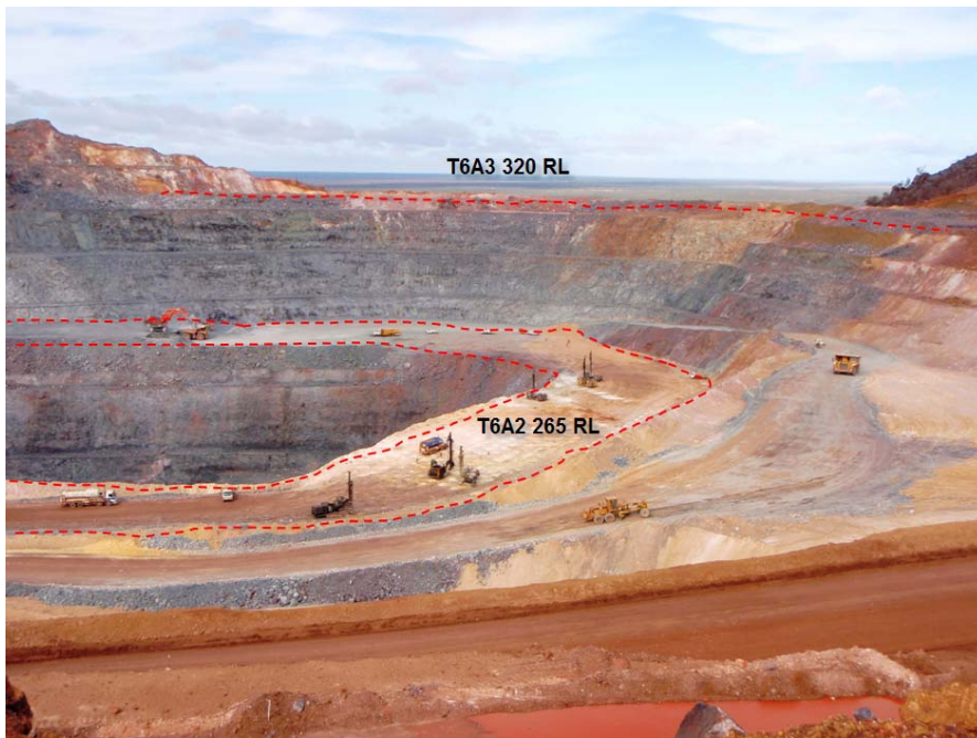
Figure 4 - T6A2 cutback from main range operation north wall
