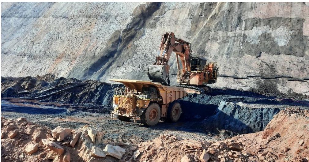
Figure 2: High-grade (65% Fe) iron ore mining, central Main Pit, April 2022.
