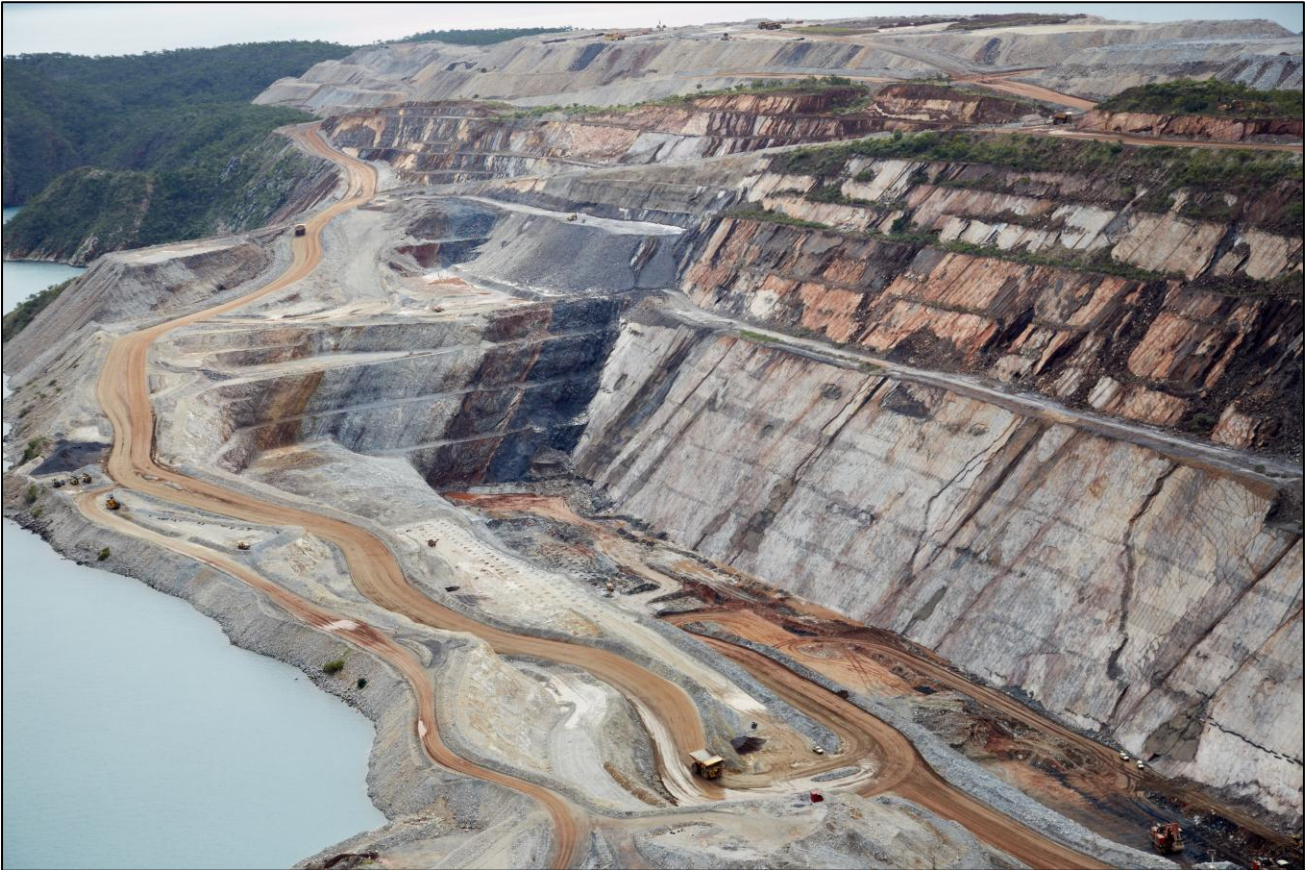
Figure 1: Mining activity in Koolan Island Main Pit, June 2013. Dark band at the end of the pit is ore.
