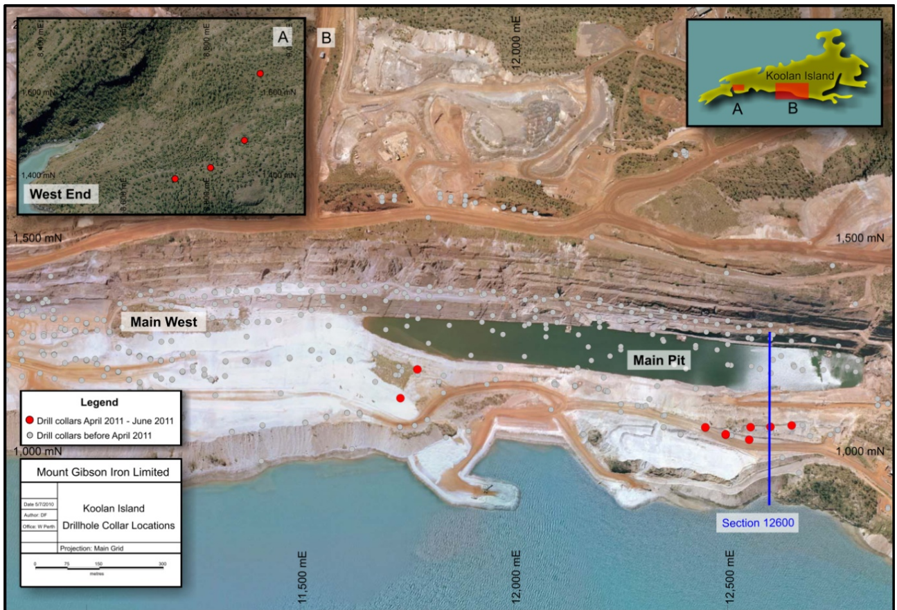
Figure 14 – Plan of Main Pit, Koolan Island showing drillhole collar locations for holes drilled during the quarter (red circles) and all previous drilling (grey)
