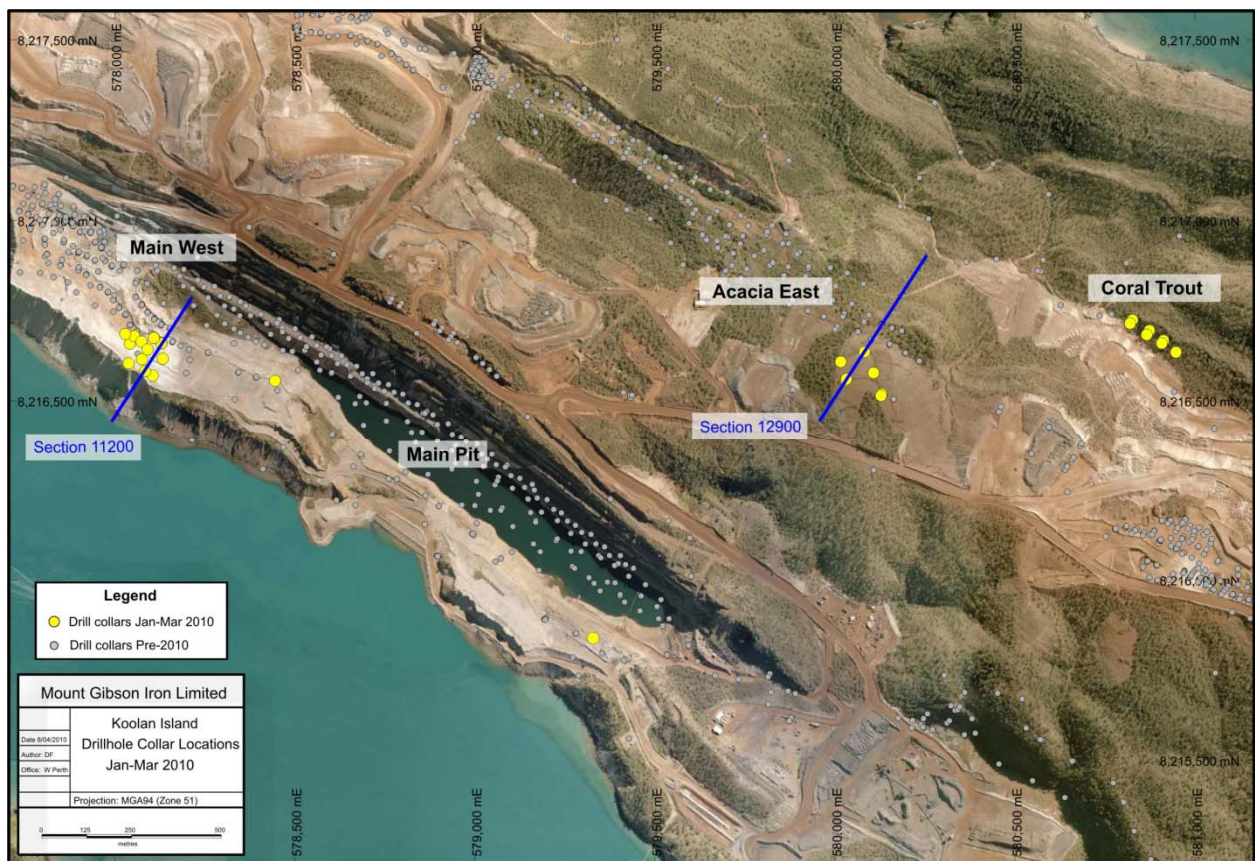
Figure 15 – Plan of Koolan Island showing drillhole collar locations for holes drilled during the Quarter (yellow circles) and all previous drilling (grey)
