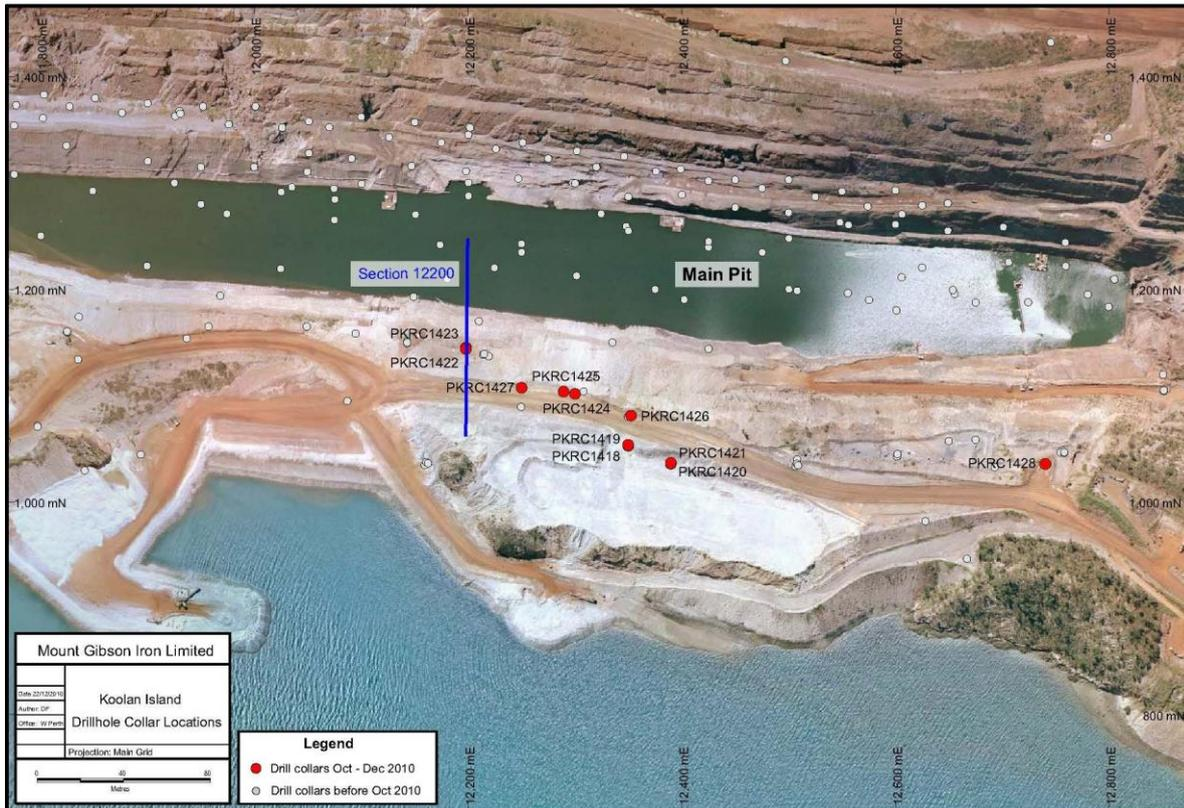
Figure 10 – Plan of Main Pit (eastern end), Koolan Island showing drill-hole collar locations for holes drilled during the quarter (red circles) and all previous drilling (grey)
